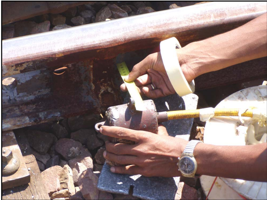
Figure 4.13. Setup of Isotope to Radiograph the Rail Web.
